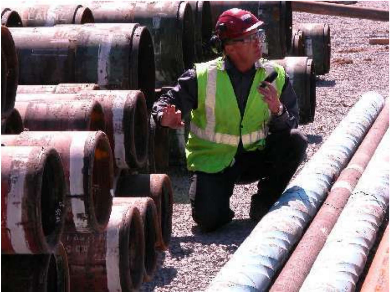
Eddie Buckley explaining the job of the casings behind him and drill string sections in front
