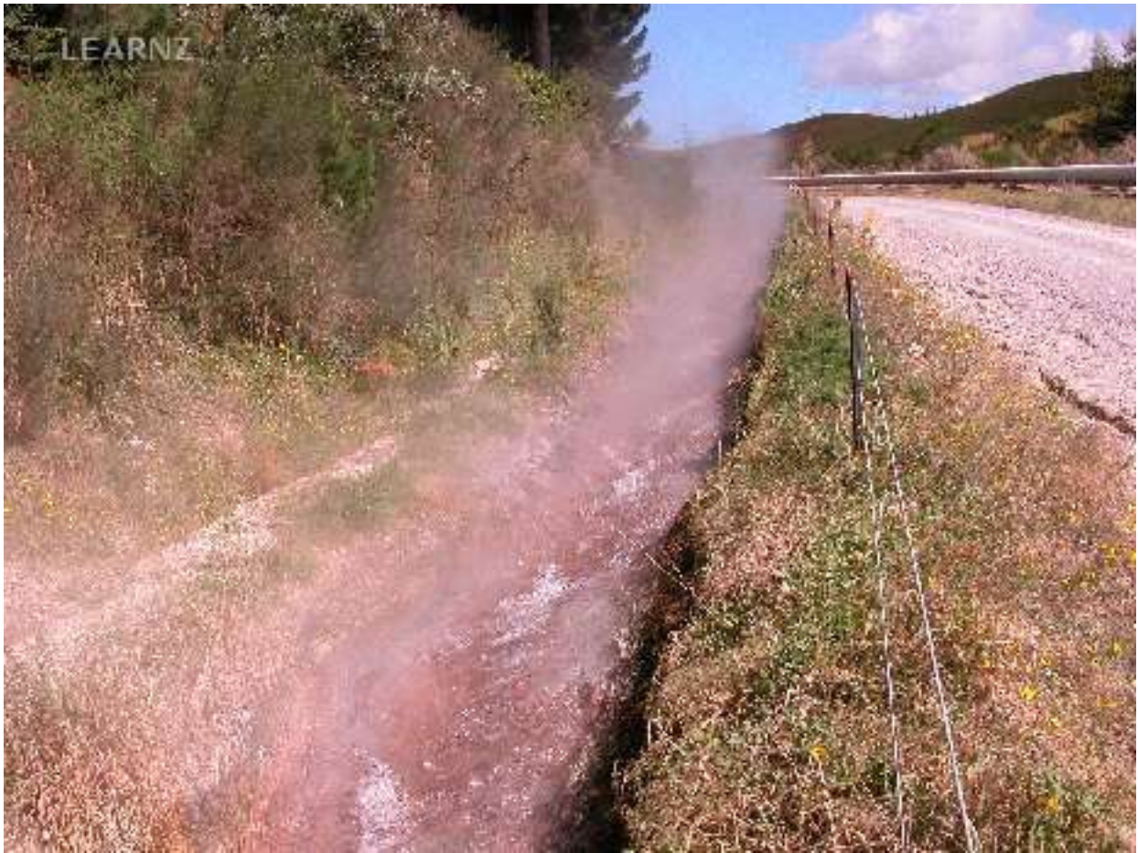
Hot water escapes from the silencer and cascades at 1000 tonnes per hour down to the Waikato River
