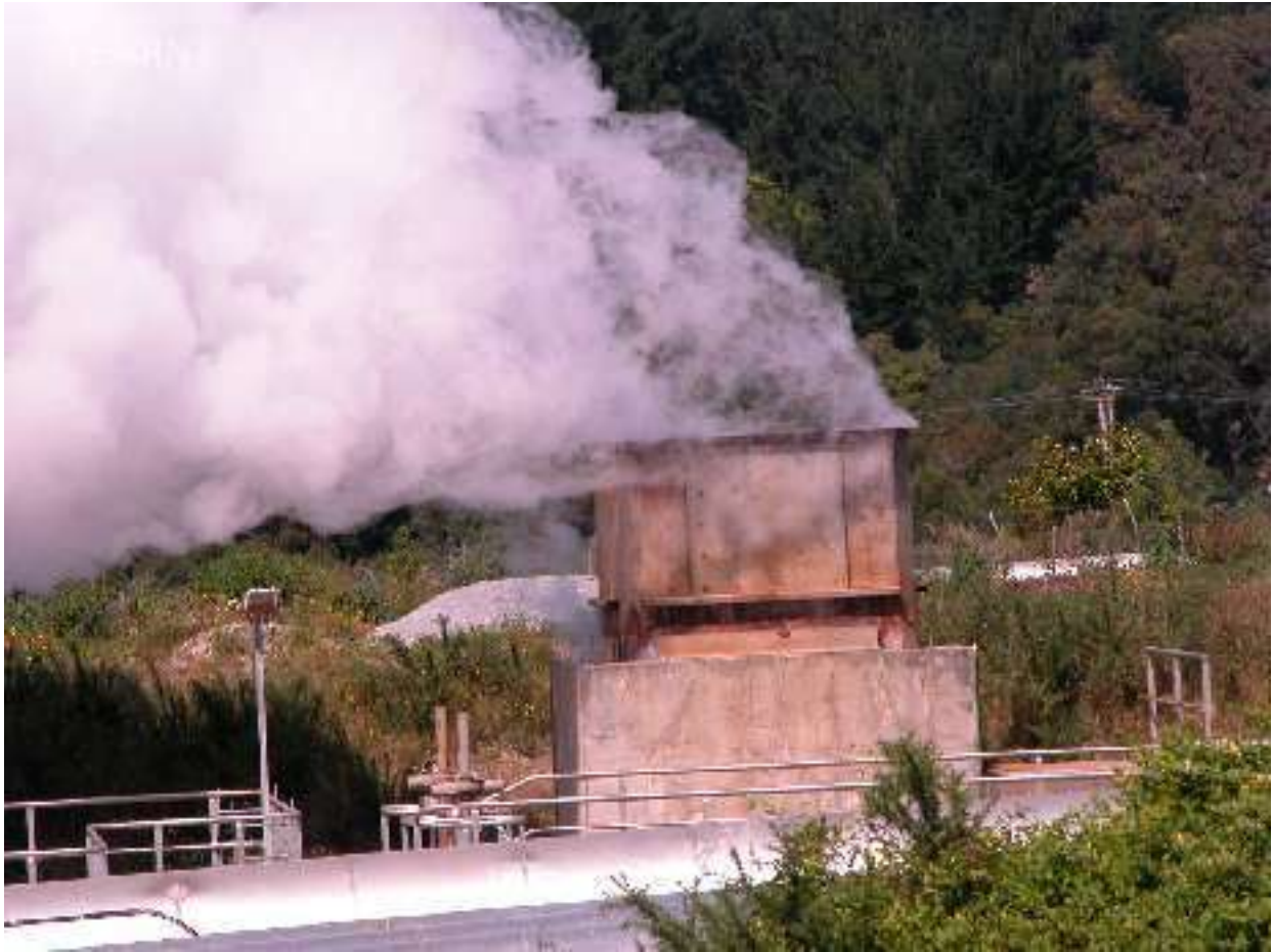
The white clouds are water vapour but the steam, just above this silencer, is colourless
