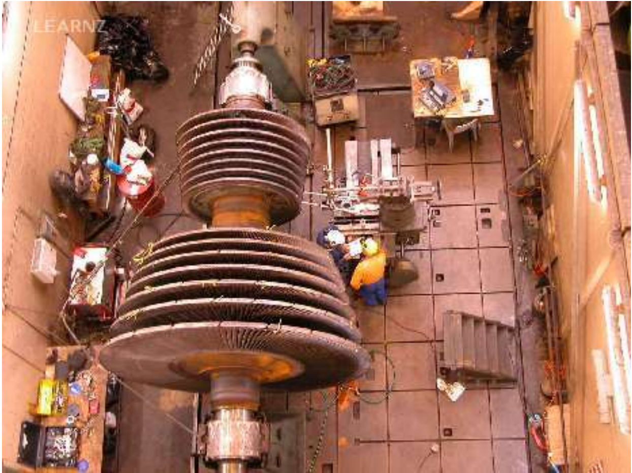
The rotor of Mixed Pressure turbine G11 sits in the lathe in the floor below undergoing inspection
