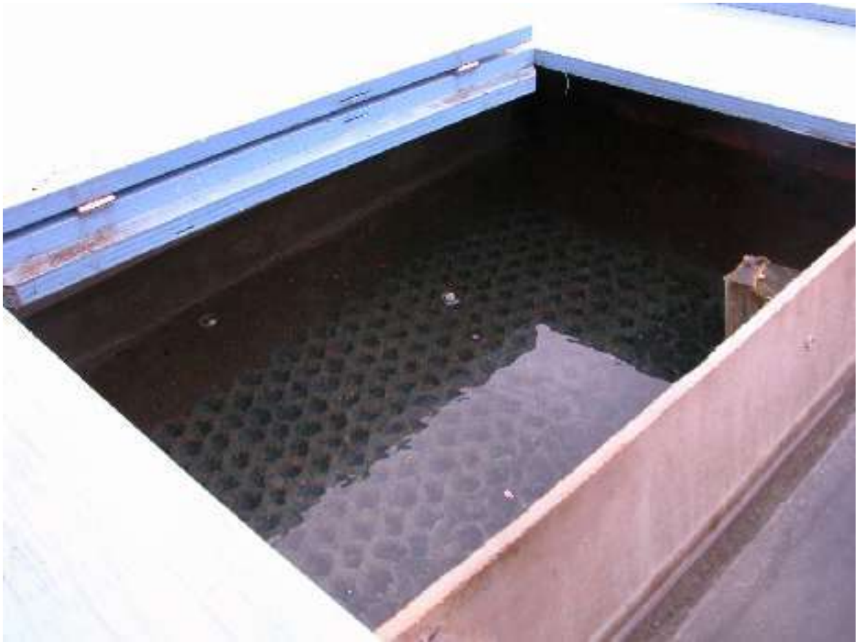
Inside the bioreactor pilot plant where grey bacteria can be seen growing profusely on the plastic screens
