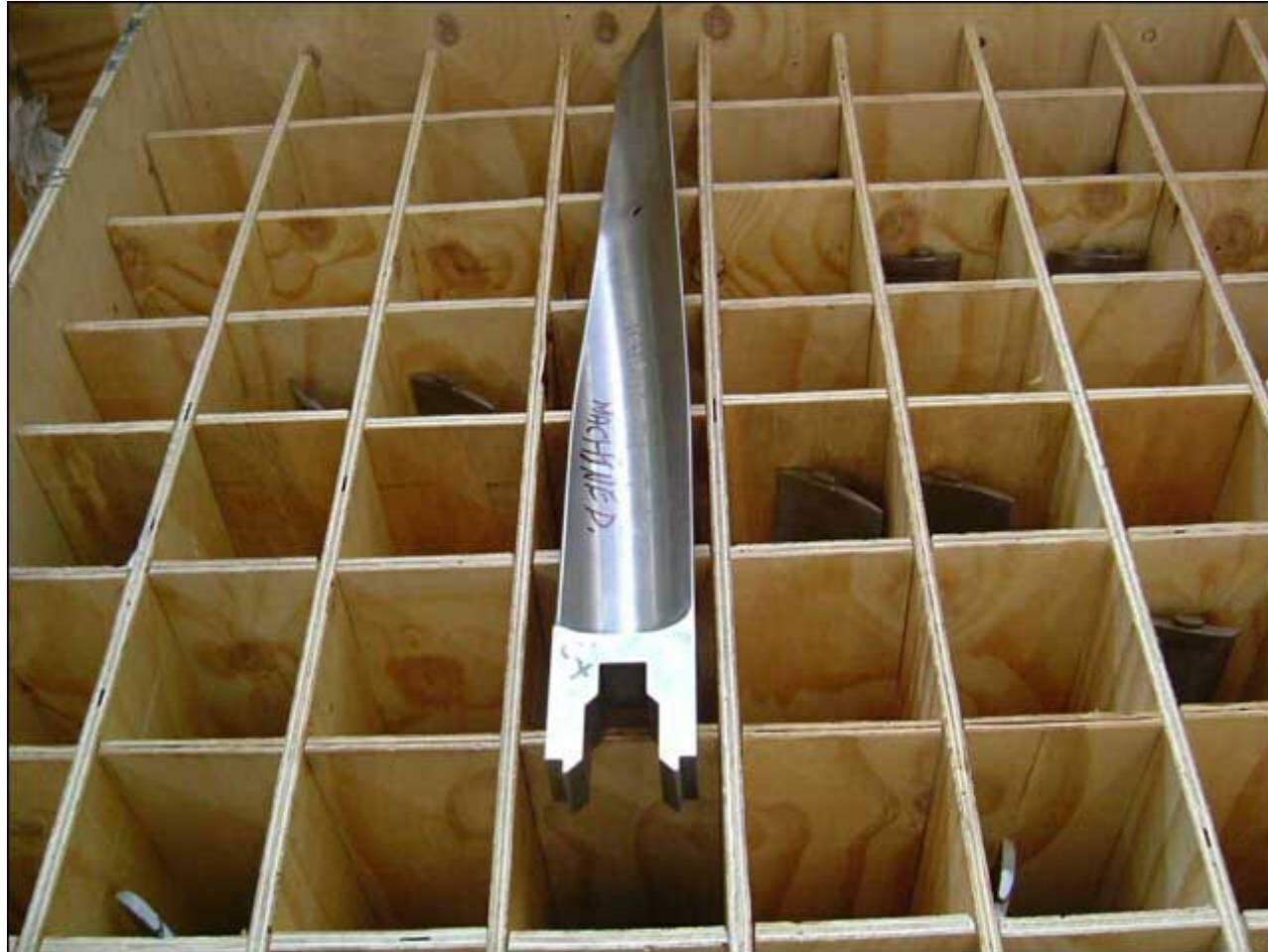
A single blade from the low-pressure steam turbine that drives Generator 9. Others are stacked below.
